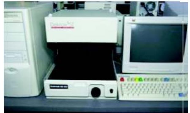
Dektek 3® – A surface profiler used by SIMCO to measure roughness and topography on substrates, polymers, optical lenses, metallurgy and advanced materials.
